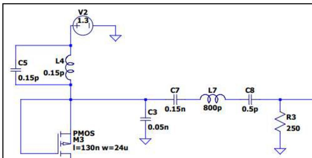
Figure 6: Part of the Class E used in the circuit
