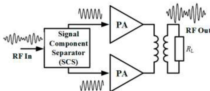
**Figure 3:** Simplified outphasing PA architecture diagram [7].
