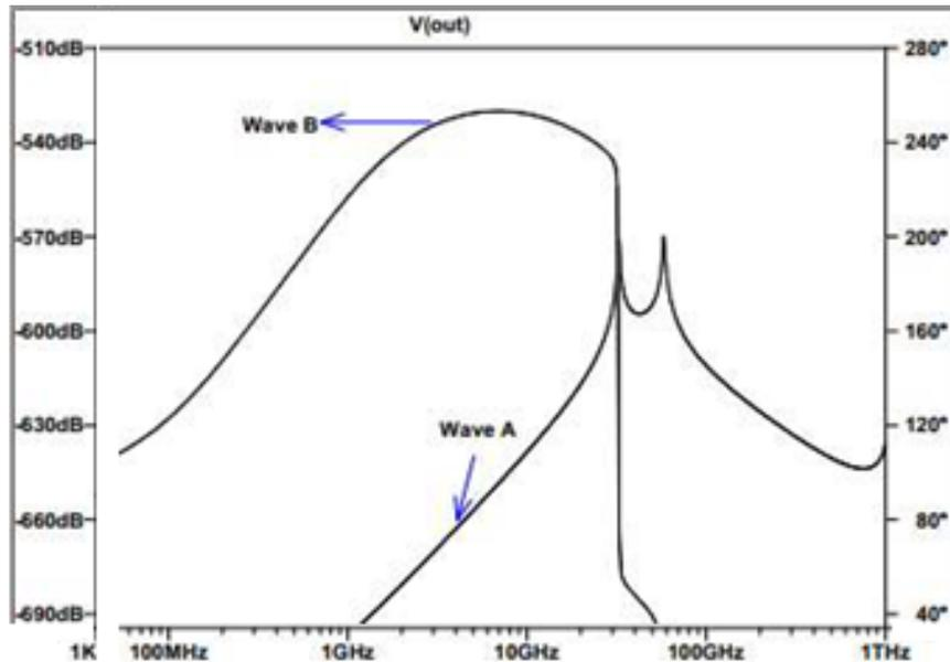
**Figure 8:** Bandwidth waveform of the outphasing PA
