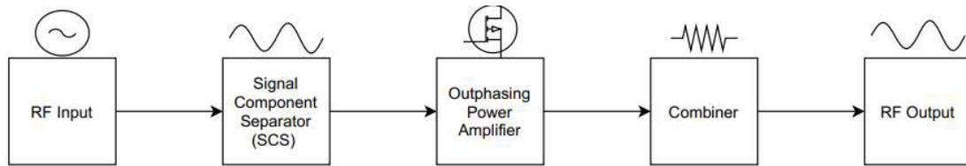
**Figure 4:** Block Diagram of the Outphasing PA.
