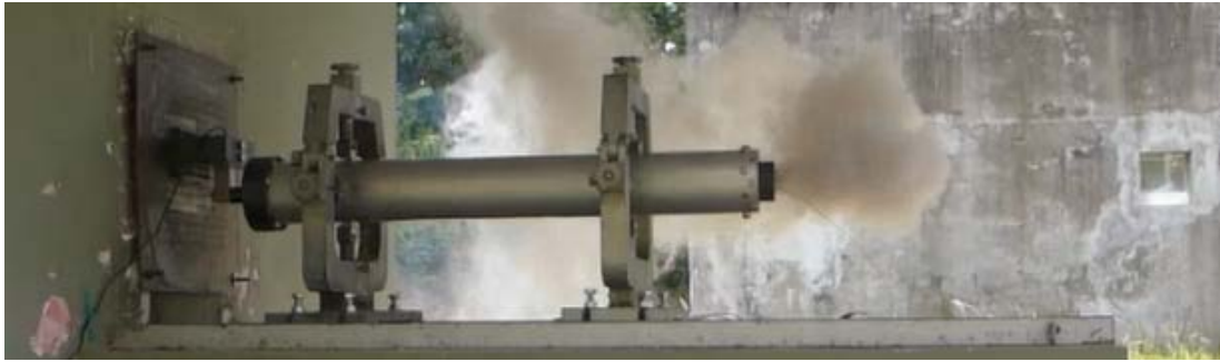
Figure 5: Initial combustion of solid rocket motor at t \approx 0.1 second.
