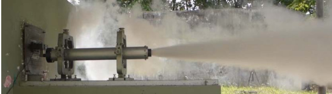
Figure 6: Combustion of solid rocket motor at t \approx 0.3 second.
