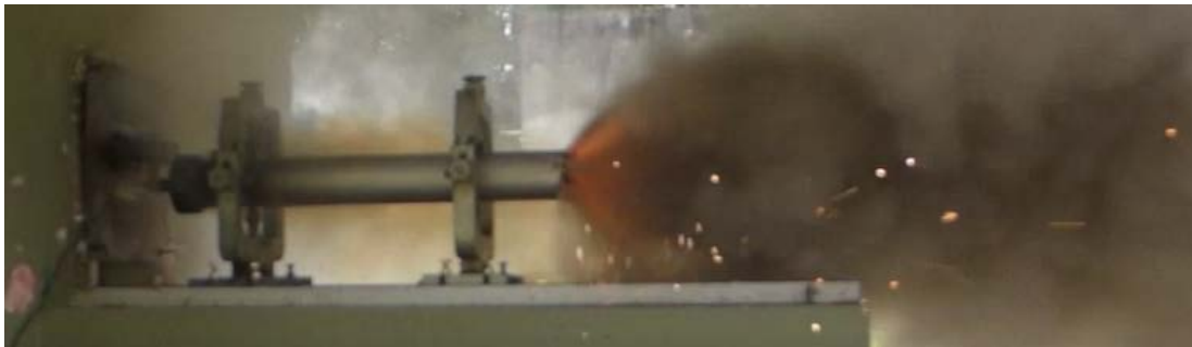
Figure 7: Combustion of solid rocket motor at t \approx 0.6 second.
