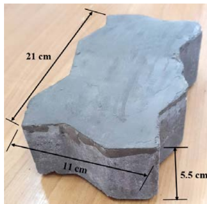
Figure 3: Interlocking paving block used in the investigation
