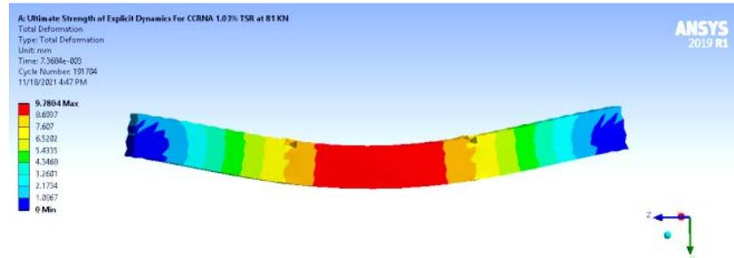
**Figure 5:** Deflection of the beam at ultimate stage.
