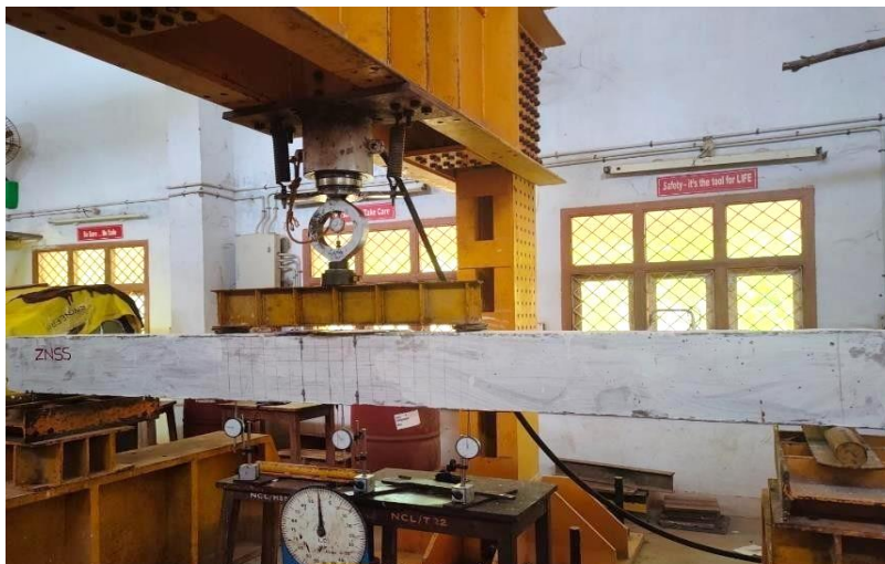
Figure 2: Static Loading Arrangement and Instrumentation
