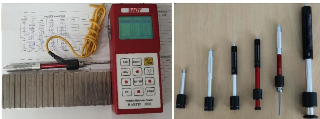
Figure 1: Portable hardness tester HARTIP 3000.
