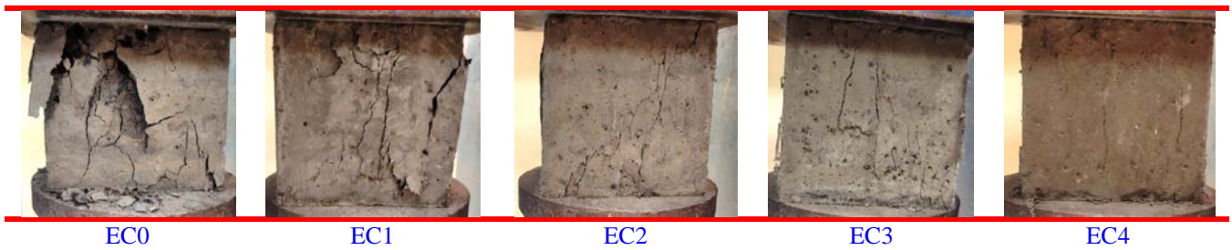
Figure 8: Failure Pattern of Cube specimens
