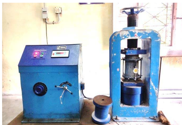
Figure 4: Elasticity Modulus Test on Cylinder
