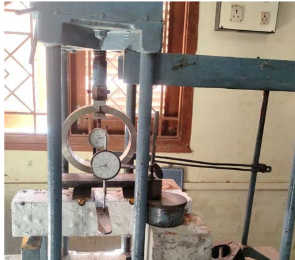
Figure 5: Flexure Test on Prism
