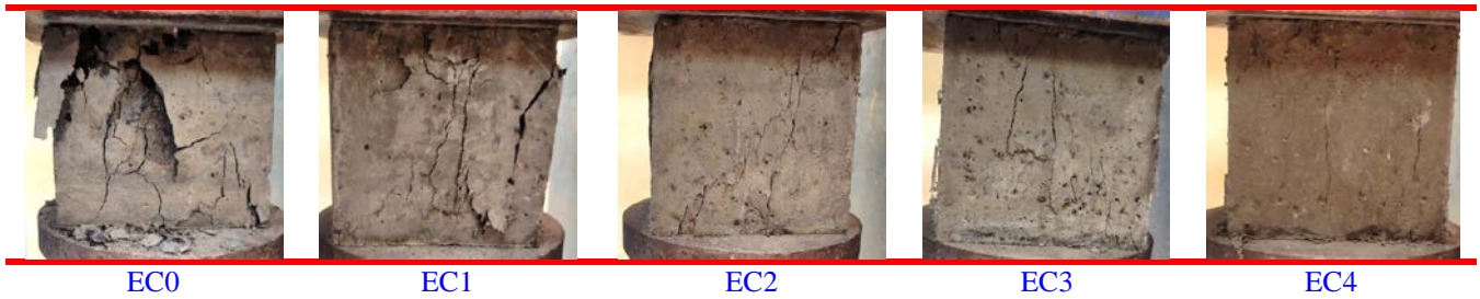
Figure 8: Failure Pattern of Cube specimens
