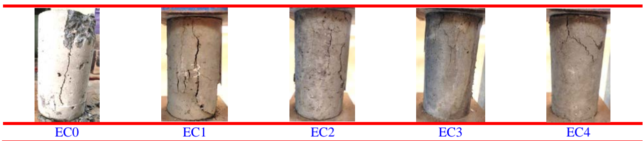
Figure 10: Failure Pattern of Cylinder Specimens
