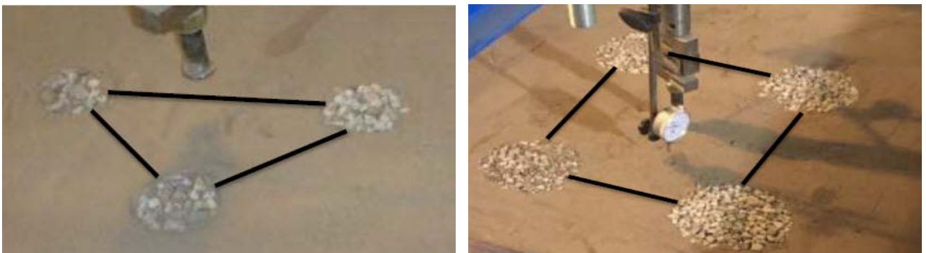
Figure 1: Display the square and Triangle arrangement of stone columns in the present article
