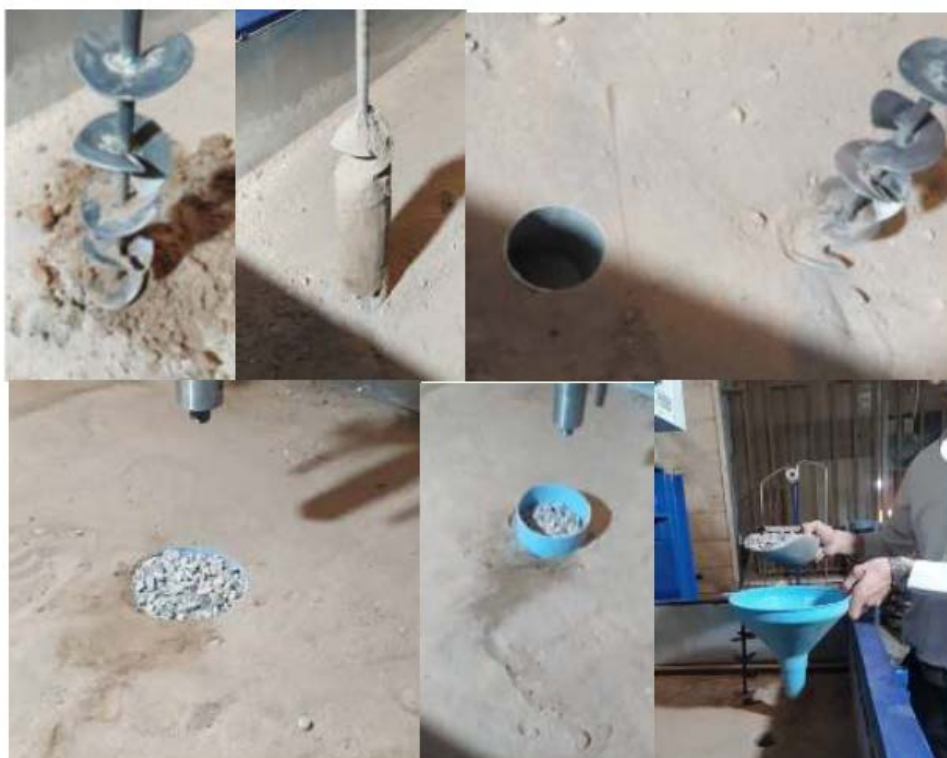
Figure 5: construction processes of stone column
