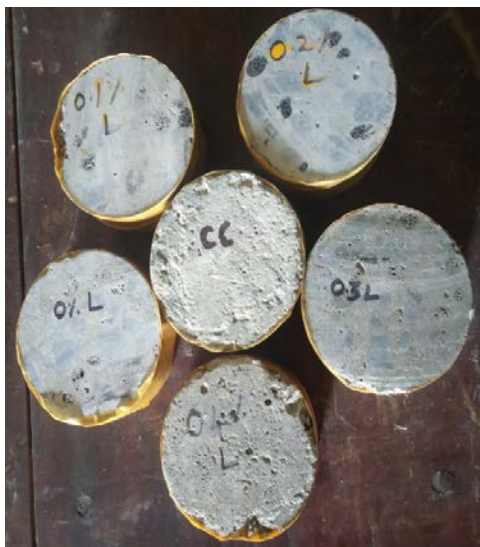
Figure 3: Disc sealed with adhesive tape
