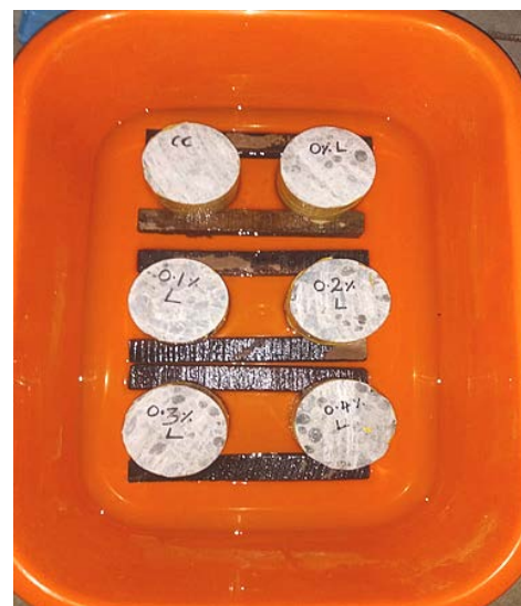
Figure 4: Sorptivity Test Setup
