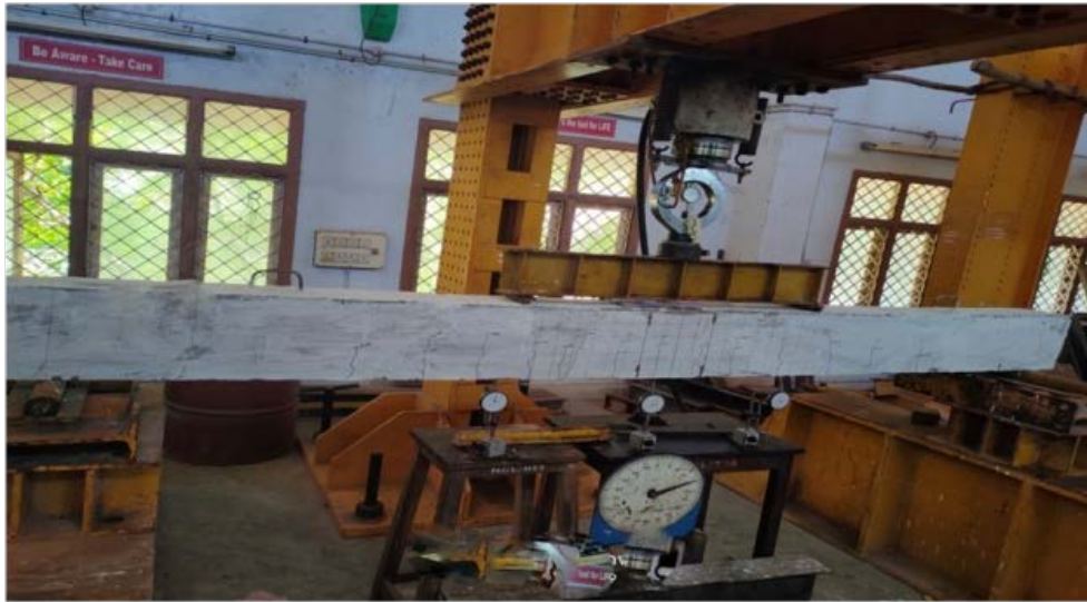
Figure 3: Static Loading Arrangement and Instrumentation
