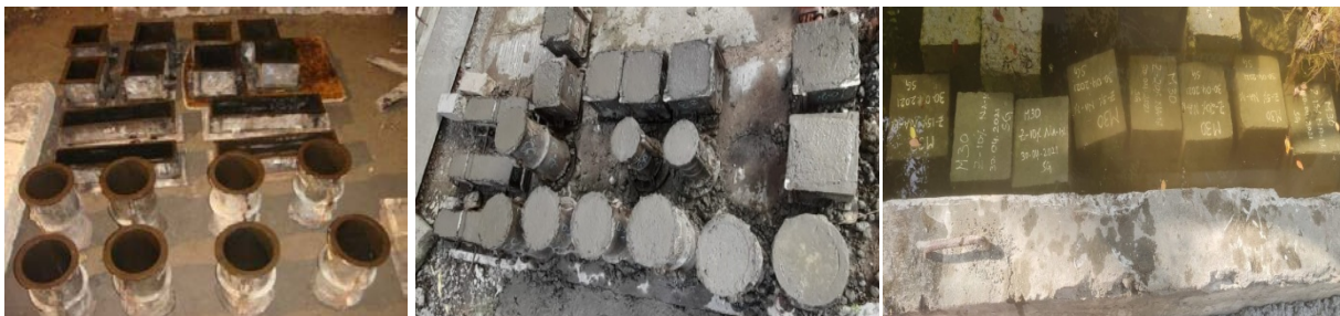
Figure 1: Casting and Curing of Control Specimens
