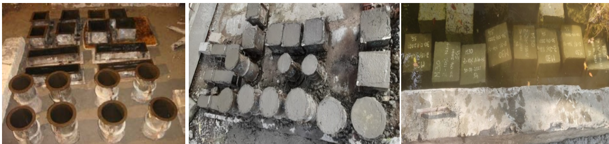
Figure 1: Casting and Curing of Control Specimens
