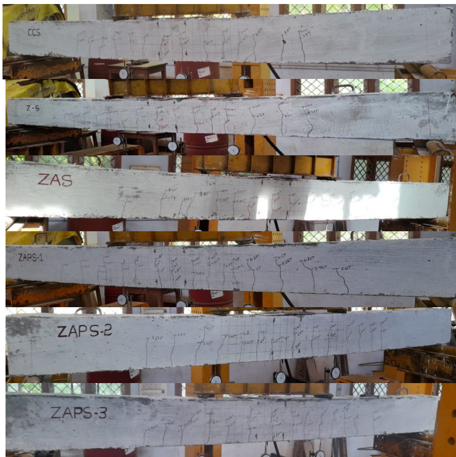
Figure 14: Crack Pattern of Beam Specimens
