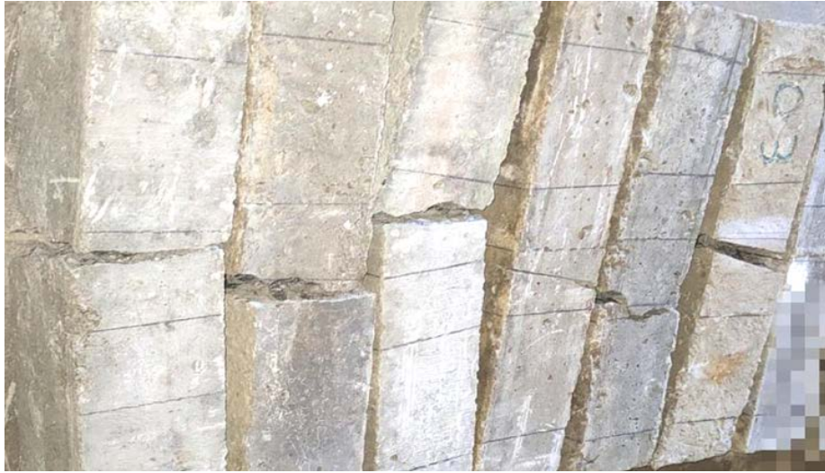
Figure 10: Failure Mode of Prism Specimens
