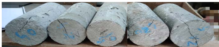
Figure 7: Failure Mode of Cylinder Specimens Under Indirect Tension
