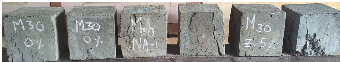
Figure 5: Failure Mode of Cube Specimens
