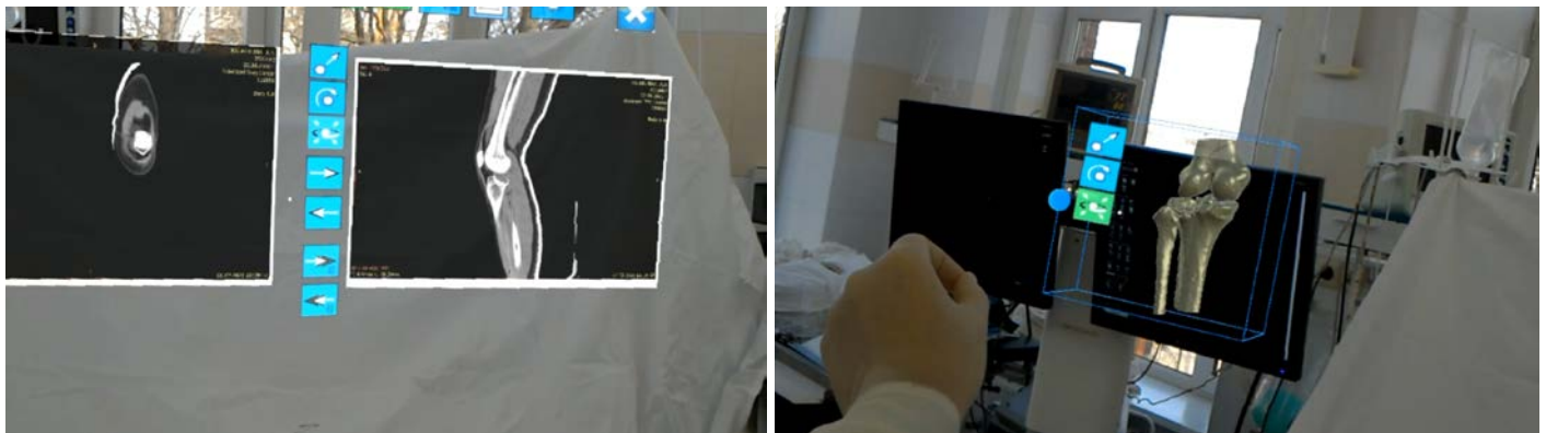
Figure 5: Viewing and navigation in augmented reality glasses HoloLens 3D reconstruction and Dicom images
