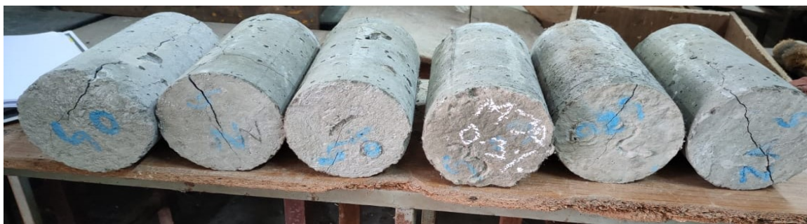
Figure 14: Failure Pattern of Cylinder Specimens
