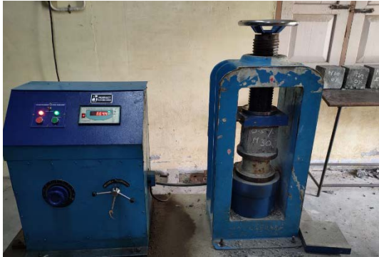
Figure 5: Cube Compressive Strength Test
