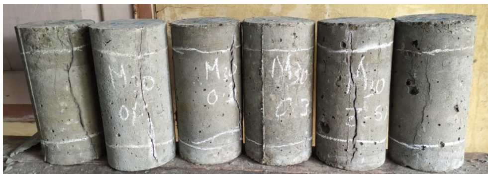
Figure 18: Failure Pattern of Cylinder Specimens.
