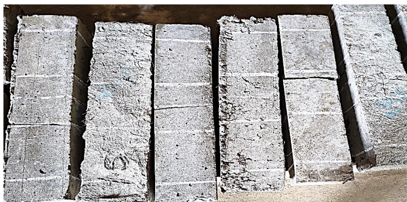
Figure 16: Failure Pattern of Prism Specimens
