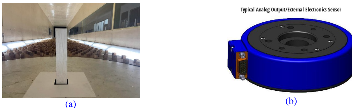
Figure 4: (a) HFFB model (b) The JR3 multi-axis load cell.
