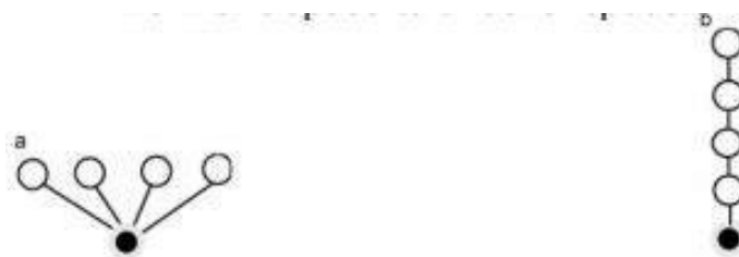
Figure 1: An elementary representation for space syntax analysis- "a" represents minimum depth ( symmetric system), "b" a linear sequence of maximum depth ( asymmetrical system)
