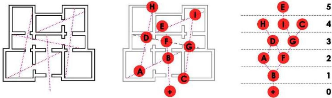
**Figure 1:** Level of Depth in Space Syntax Redrawn by author
